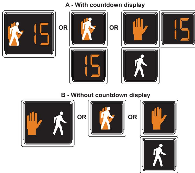
Figure 4E-1. Typical Pedestrian Signal Indications
