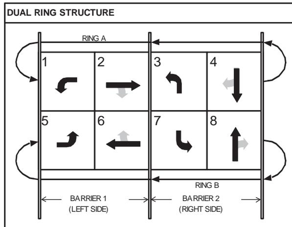
The dual-ring controller uses a maximum of eight phase modules, each of which controls a single traffic signal face with red, yellow and green display. The eight phases are required to accommodate the eight movements (four through and four left turns) at the intersection. Phases 1 through 4 are included in ring 1, and phases 5 through 8 are included in ring 2. The two rings operate independently, except that their control must cross the “barrier” at the same time.
