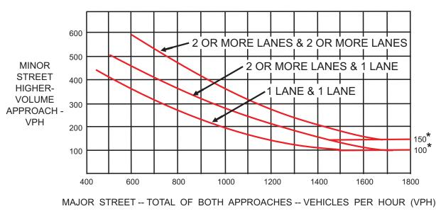
\*NOTE: 150 vph applies as the lower threshold volume for a minor-street approach with two or more lanes and 100 vph applies as the lower threshold volume for a minor-street approach with one lane.
