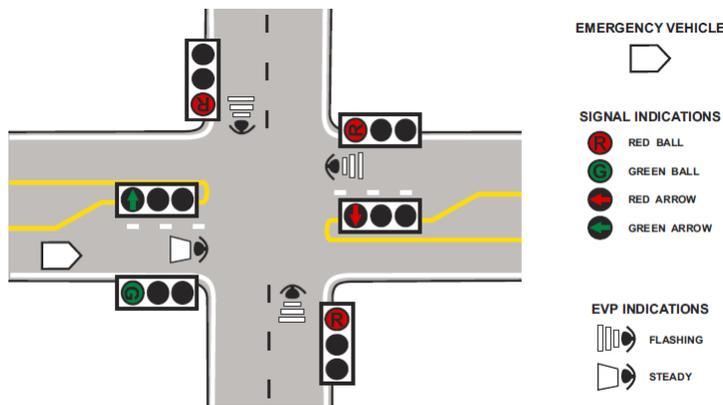
Figure 4D-24. Emergency Vehicle Preemption (EVP) - Protected Operation
