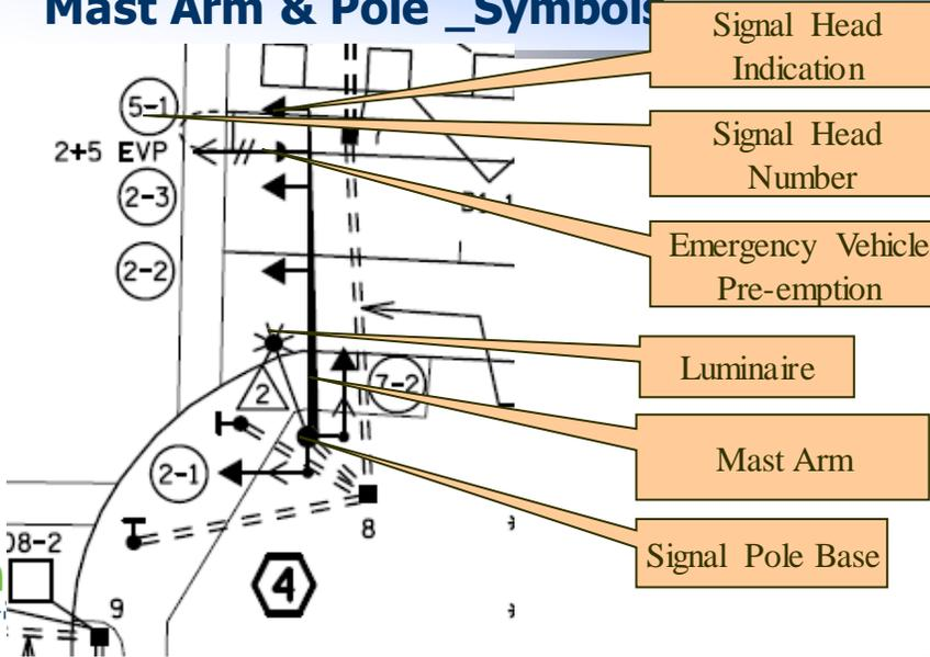
The signal bases and pole notes are shown in a hexagon. The signal bases are labeled clockwise around the intersection with Number 1 being adjacent to or near the controller cabinet.
