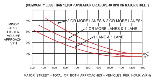
\*NOTE: 100 vph applies as the lower threshold volume for a minor-street approach with two or more lanes and 75 vph applies as the lower threshold volume for a minor-street approach with one lane.
