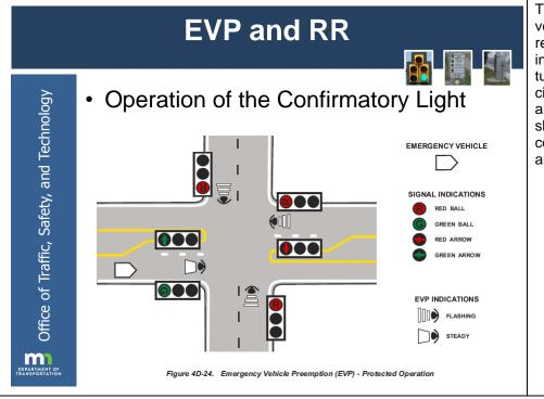
The authorized emergency vehicle's approach shall receive a steady confirmatory indicator light, a protected left turn green arrow, and a circular green. The opposing and conflicting approaches shall receive flashing confirmatory indicator lights and red indications.
