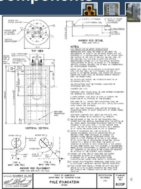
This is Standard Plate No. 8120, Pole Foundation for a type PA85. Standard Plate No. 8126 is for foundation PA90 and PA100 (longer mast arms) and 8133 is for Type BA. See page 3-5 for information on mast arm lengths). Refer to the Standard Plates for the most current version.
