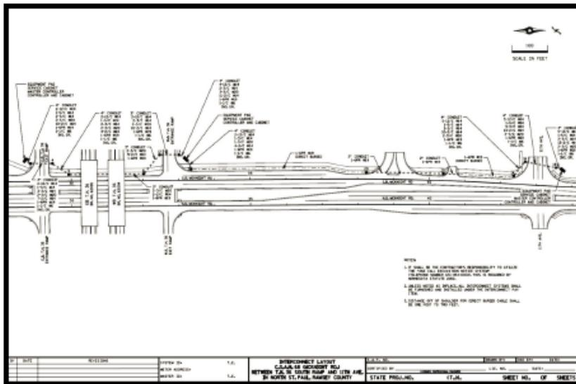
This plan sheet shows interconnect for the project. Interconnect is a means of remotely controlling some or all of the functions of a traffic signal. It also allows the master controller to communicate with any local controllers in the system.
