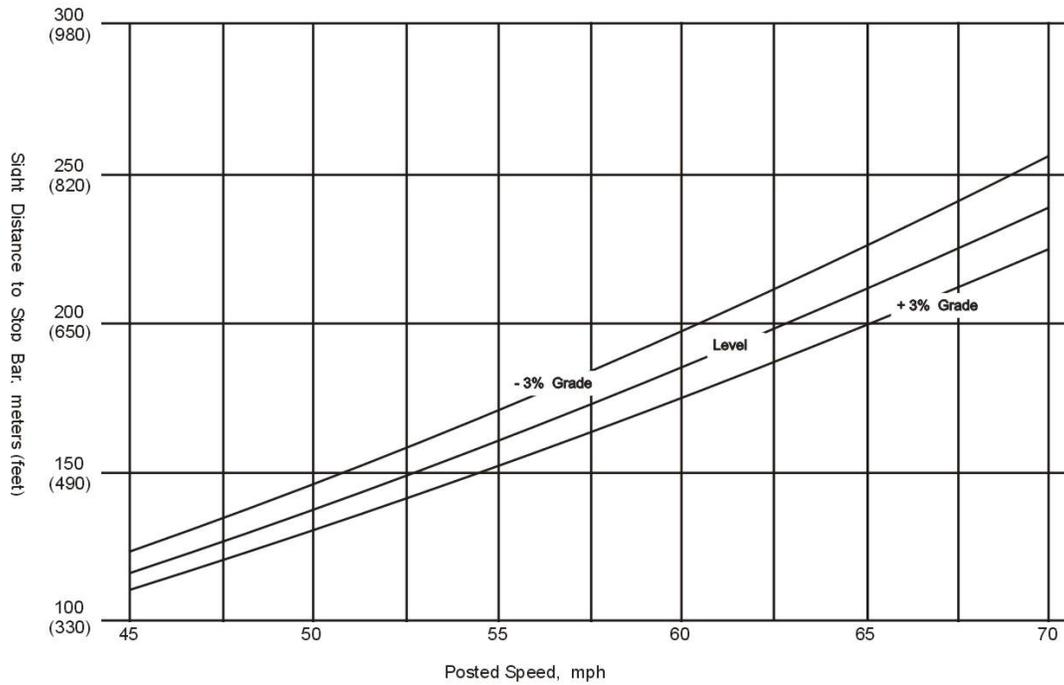
A sight distance falling below the lines for the given speed and grade indicates the possible need for an AWF.
