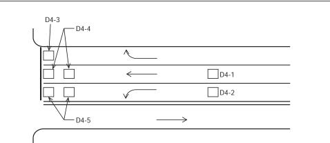
LOCATION = DISTANCE FROM STOP BAR TO LOOP DETECTOR
