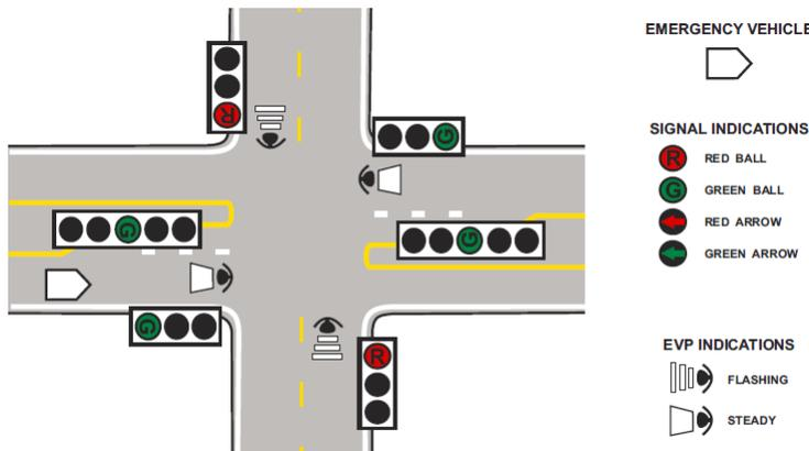
Figure 4D-22. Emergency Vehicle Preemption (EVP) - Protected/Permissive Operation
