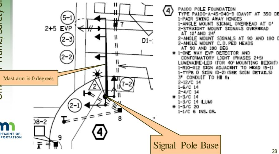
These are the signal pole notes. The mast-arm is at 0 degrees. Items referenced with angles are in relation to the mast arm pole in the clockwise direction.
