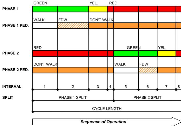
For the figure to the left, there are eight intervals where the signal indications do not change. Notice that intervals 4 and 8 are all red periods (interval 4 is the phase 1 all red and interval 8 is the phase 2 all red). The phase 1 split is made up of intervals 1 through 4 and the phase 2 split is made up of intervals 5 through 8. The sum of split 1 and 2 is the cycle length.
