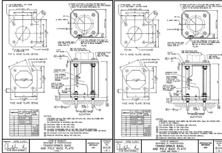
This is Standard Plate No. 8121 (page 1 and 2), Transformer Base and Pole Base Plate.
