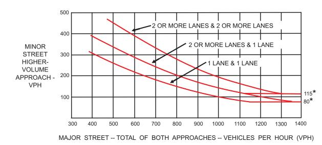
\*NOTE: 115 vph applies as the lower threshold volume for a minor-street approach with two or more lanes and 80 vph applies as the lower threshold volume for a minor-street approach with one lane.
