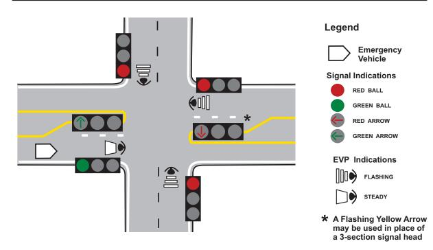
Figure 4D-24. Emergency Vehicle Preemption (EVP) - Protected Operation
