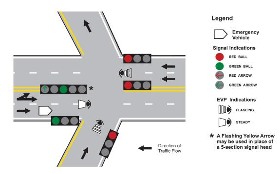
Figure 4D-23. Emergency Vehicle Preemption (EVP) -Ramp/One-Way/T-Intersection Protected/Permissive Operation
