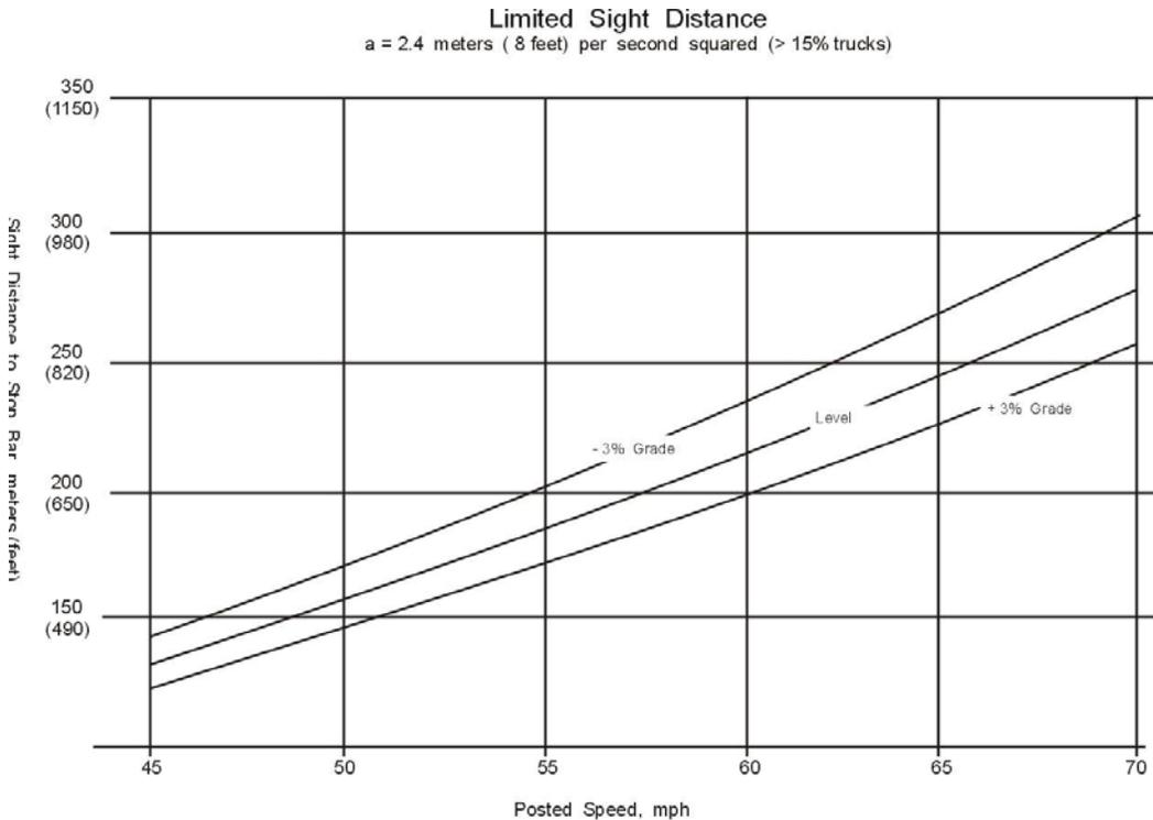
A sight distance falling below the lines for the given speed and grade indicates the possible need for an AWF.
