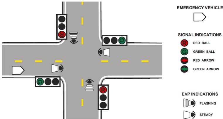
Figure 4D-21. Emergency Vehicle Preemption (EVP) - Two Phase Operation
