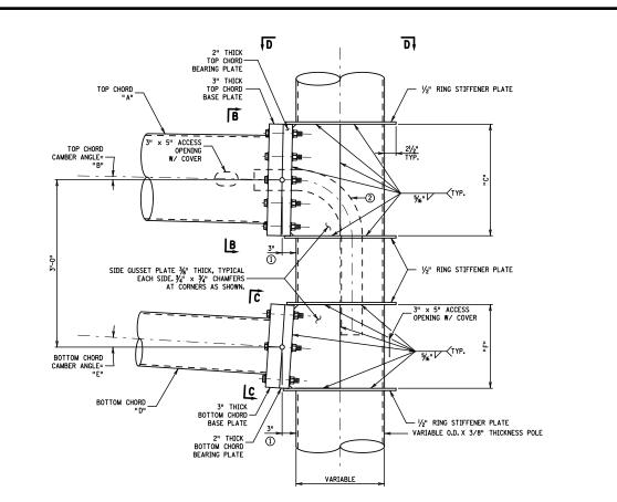
DETAIL B MAST ARM CONNECTION DETAILS
