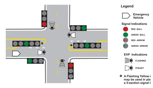
Figure 4D-22. Emergency Vehicle Preemption (EVP) - Protected/Permissive Operation
