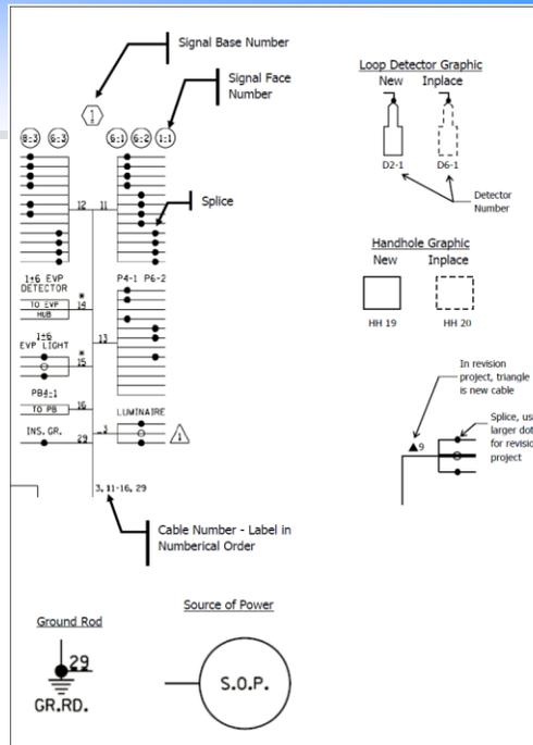
The field wiring diagram is used to describe how the actual field wiring shall be placed.
