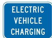
D9-11bP Electric Vehicle Charging
