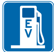
D9-11b Electric Vehicle Charging
