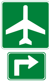
Example of direction assembly
