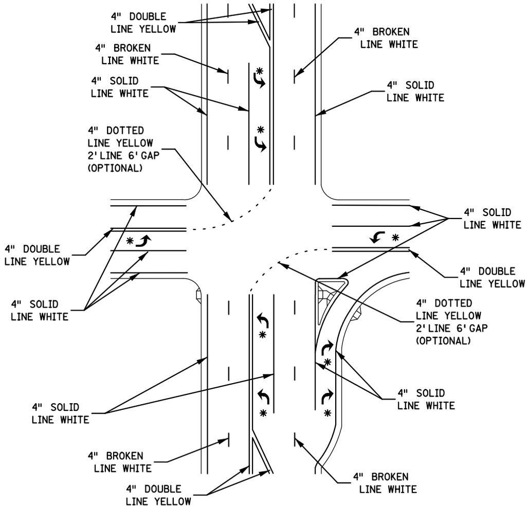
DESIGNER'S NOTES: CENTER LINE EXTENSIONS IN THE INTERSECTION SHALL BE 4" DOTTED YELLOW LINES. TYPICAL PAVEMENT MARKINGS WITH OFFSET LANE LINES CONTINUED THROUGH THE INTERSECTION MAY BE 4" DOTTED OR SOLID WHITE LINES.
