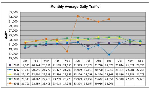
Note: Decrease in traffic July to September 2012 and May 2015 due to construction on TH 14; Increase in traffic beginning November 2012 due to an addition of two lanes at the site, and during June to September 2015 due to detours
