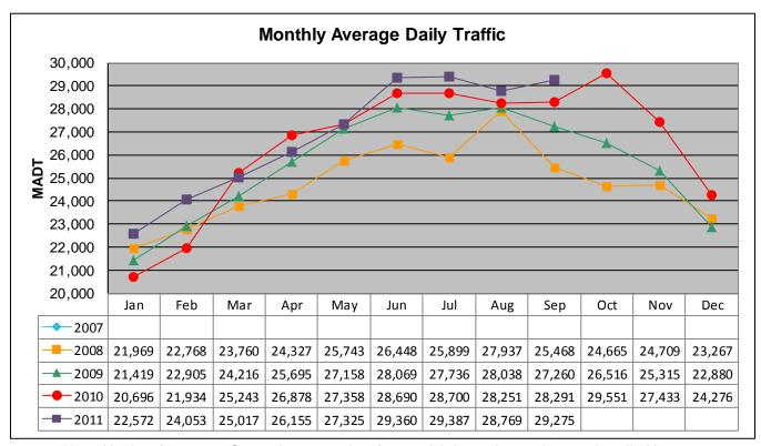
Note: No data for 2007... Currently reports data from weigh-in-motion station #32 installed in 2008
