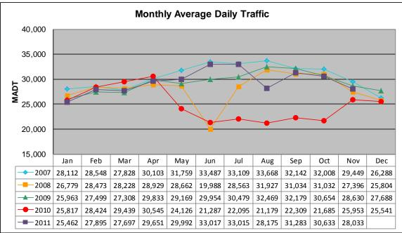
Note: Decrease in traffic June/July 2008 due to bridge work... Decrease in traffic May to October 2010 and August 2011 due to construction on I-35
