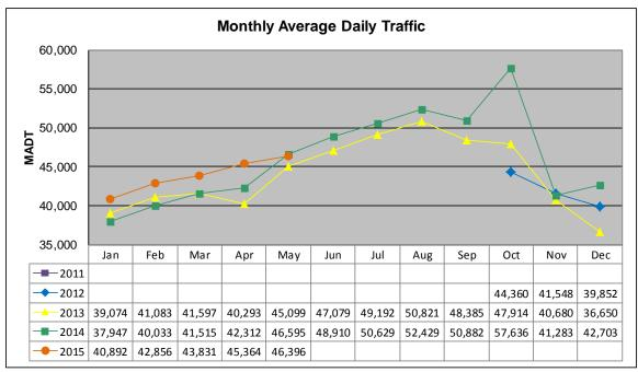
Note: No data from January 2011 to September 2012 due to sensors destroyed by construction... Increase in traffic October 2014 due to detour from bridge construction
