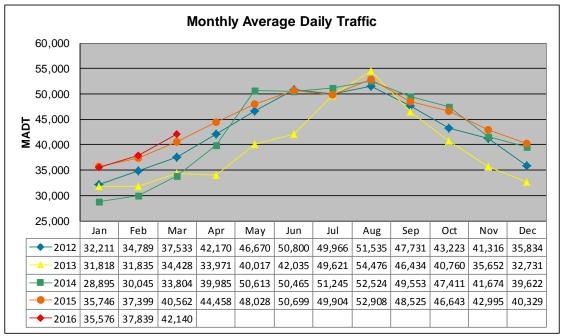
Note: Decrease in traffic April to June 2013 due to construction on I-94... Increase in traffic August 2013 and May/June 2014 due to TH 10 detours
