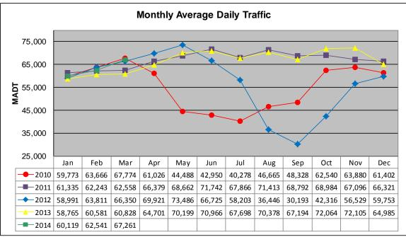
Note: Decrease in traffic April to October 2010 and June to November 2012 due to construction on I-694... Increase in traffic November 2013 due to detour from TH 36
