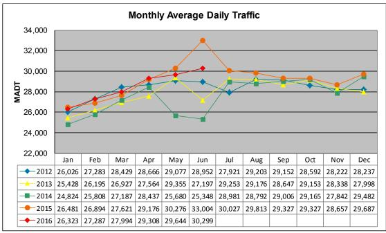
Note: Decrease in traffic June 2013 and May/June 2014 due to construction on CSAH 42... Increase in traffic June 2015 due to detours
