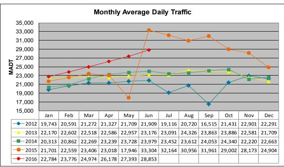
Note: Decrease in traffic Jul-Sep 2012 and May 2015 due to construction on TH 14... Increase in traffic beginning Nov 2012 due to an addition of two lanes at the site, and during Jun-Dec 2015 and Apr-Jun 2016 due to detours
