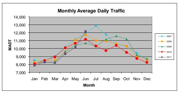
Note: Increase in traffic July 2007 due to detour from I-694 & I-35E and June 2011 due to detour from I-35E... Decrease in traffic August/September 2010 due to construction on TH 61
