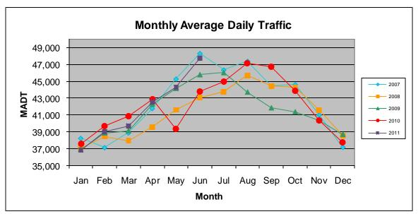
Note: Decrease in traffic 2008-2009 due to I-35W bridge collapse and construction ... Decrease in traffic May to July 2010 due to construction on I-35W and TH 62
