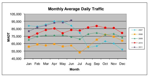
Note: Decrease in traffic 2007-2008 due to I-35W bridge collapse and construction on TH 62... Although traffic increased from 2008 to 2010, volumes were lower than expected due to construction on I-35W and TH 62
