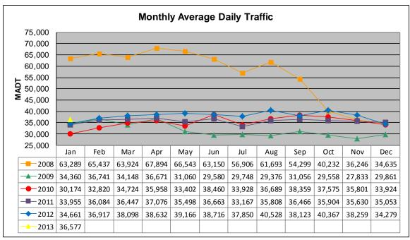
Note: Increase in traffic January to August 2008 due to I-35W bridge collapse and detour ... Traffic returned to expected volume October 2008 due to reopening of I-35W bridge
