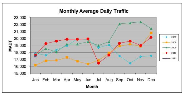
Note: Decrease in traffic July to October 2007 and July to November 2010 due to construction on TH 61... Addition of a parallel route kept traffic relatively low through November 2008
