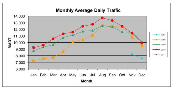
Note: No data January to October 2007 due to sensors destroyed by construction... Increased traffic beginning August 2008 due to new TH 212 being opened
