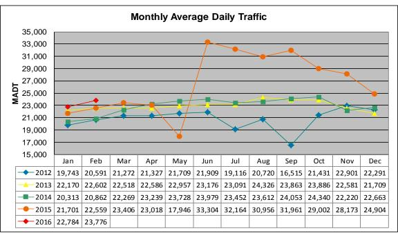
Note: Decrease in traffic July to September 2012 and May 2015 due to construction on TH 14... Increase in traffic beginning November 2012 due to an addition of two lanes at the site, and during June to December 2015 due to detours
