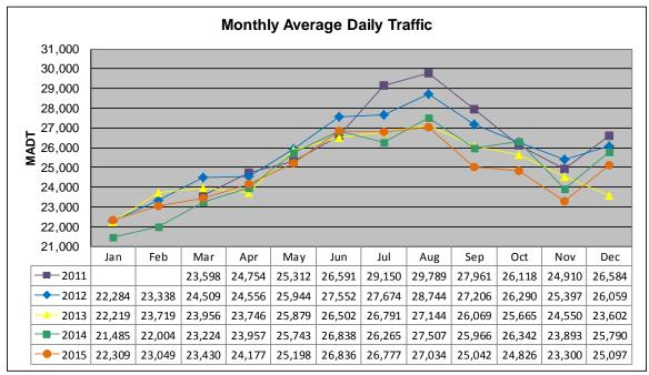
Note: No data January/February 2011 due to sensors destroyed by construction
