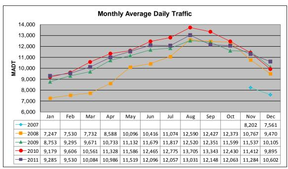
Note: No data January to October 2007 due to sensors destroyed by construction... Increased traffic beginning August 2008 due to new TH 212 being opened
