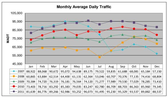
Note: Decrease in traffic 2007-2008 due to I-35W bridge collapse and construction on TH 62... Although traffic increased from 2008 to 2010, volumes were lower than expected due to construction on I-35W and TH 62
