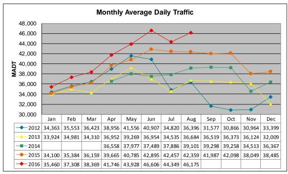
Note: Decrease in traffic July to November 2012 and June to October 2013 due to construction on TH 36... Increase in traffic June/July 2015 due to detours... No data January to March 2014 due to site communication issues
