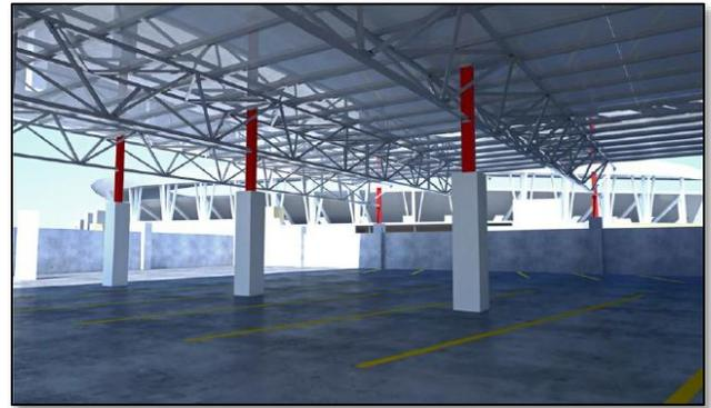
Figure 3: Design Visualization of CSG canopy on Ramp A
