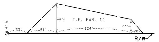
3. When Access Control and T.E. are dimensioned in the same area, all distances will be shown along the R/W line between two B-corners;
