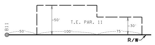
**b)** Dimension along the plat boundary, preferably along the outside of the plat boundary. As a last resort, dimensions can be placed along the outside of the T.E. and B.R.E.;
