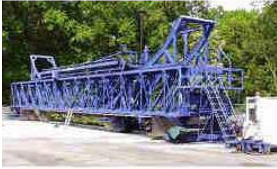
Figure 3: FHWA Accelerated Loading Facility
