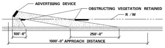
UNOBSTRUCTED VIEWING DISTANCES MAY BE ALL ONE CONTINUOUS SEGMENT OR BE DIVIDED INTO TWO SEGMENTS WITH NO LESS THAN 100 FEET IN EITHER SEGMENT
