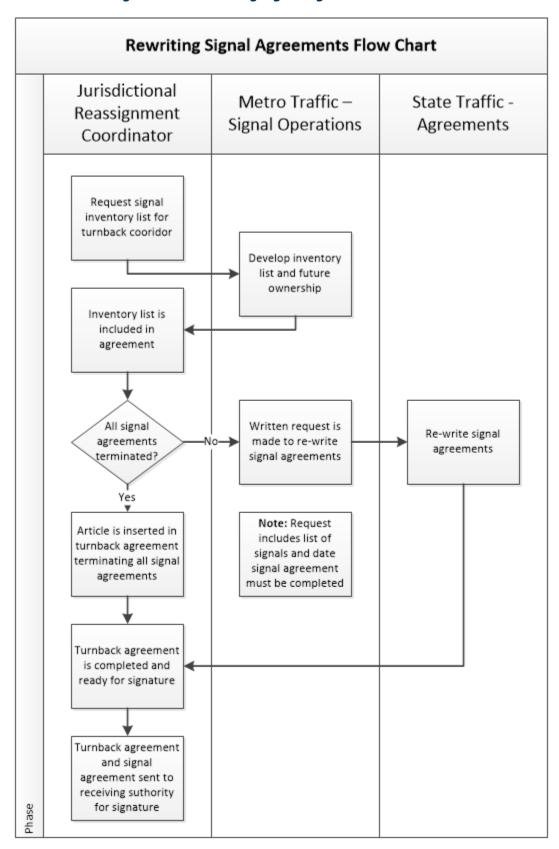
Figure 128C Turnback Process Flow Chart
