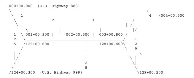
One of the routes (in this example, U.S. 888) is chosen as the "base route". The reference posts physically placed along the roadway are for the base route. The base route is stored in the usual manner with no indication of coincidence:
