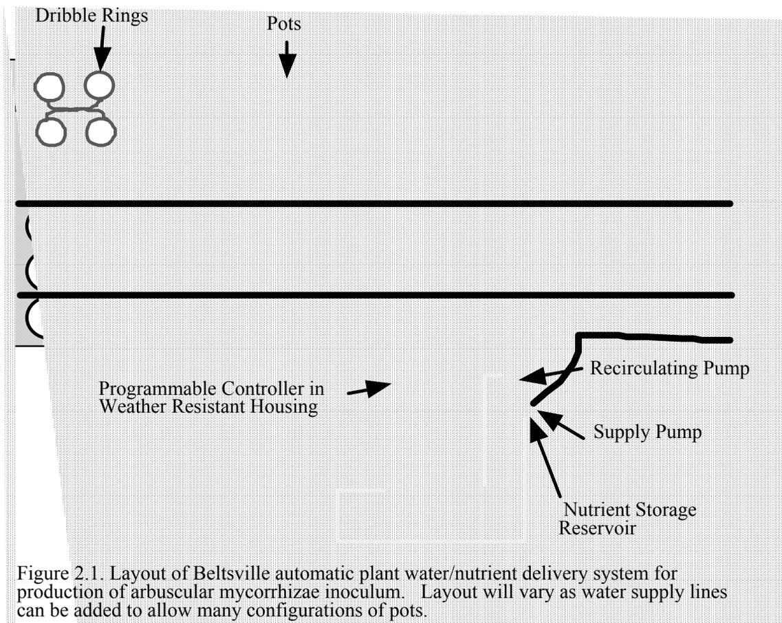
Figure 2.1. Layout of Beltsville automatic plant water/nutrient delivery system for production of arbuscular mycorrhizae inoculum. Layout will vary as water supply lines can be added to allow many configurations of pots.
