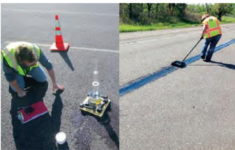
**Left:** A researcher conducts an on-site permeability test to determine how well a pothole repair seals and resists water penetration.
