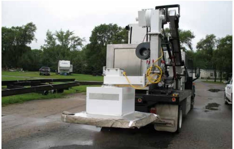
When applying a taconite-based mixture, this truck-mounted microwave unit heats both the pavement and the new patching material, creating a durable bond between pavement and fill.
