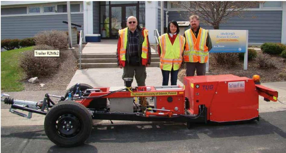
Researchers at the Technical University of Gdańsk, Poland, developed a trailer that measures rolling resistance using sensors to account for confounding variables like ride quality and slope.
