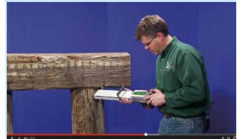
Hundreds of Minnesota timber bridges are nearing the end of their life span. To help ensure safety, inspectors are using new, high-tech tools such as stress wave timers and resistance microdrills to detect internal decay.
