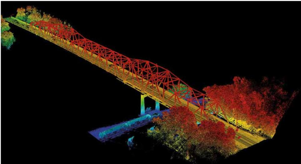
LiDAR imagery such as this image of the Highway 63 bridge in Red Wing provides survey-grade data.
