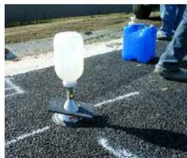
Researchers used a field permeameter to measure the hydraulic conductivity of HMA cells, or how well they allowed water to pass through them. The conductivity of porous cells decreased over time, possibly because they were becoming clogged with debris.
