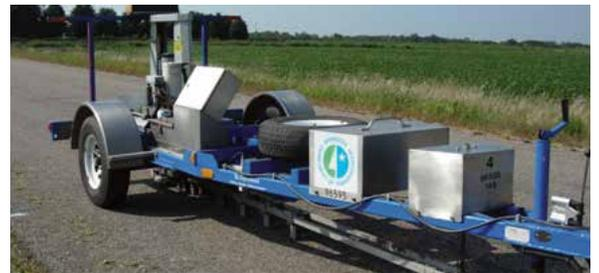
**Carried on a trailer, a falling weight deflectometer measures pavement response to loads.**
