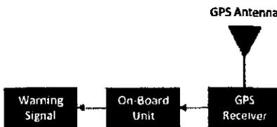
Figure 3: Block diagram of the proposed lane departure and advanced curve speed warning system.
