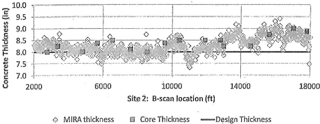
Figure 1. Use of ultrasound tomography to provide additional thickness information between cores.
