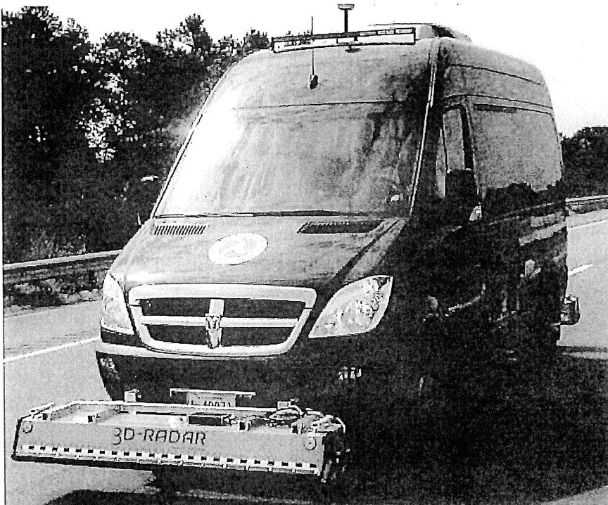
Figure 2. Advanced pavement evaluation (APE) van, retrofit with 3D Radar GPR antennae array.
