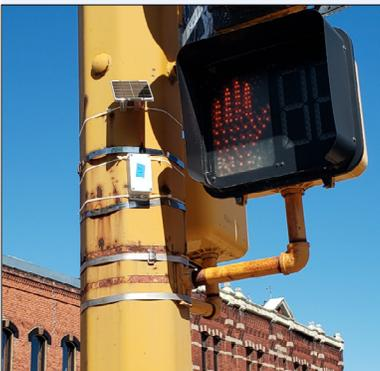
BLE beacons were installed on traffic signal poles at test sites in Stillwater, Minnesota.
