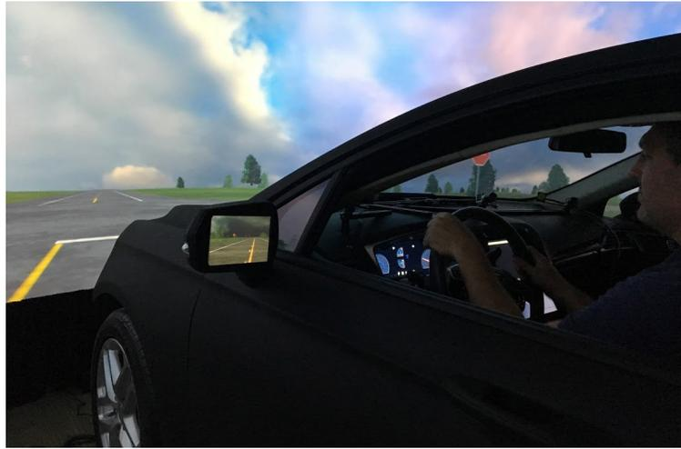
This view of the driving simulator shows the Ford Fusion cab facing one of the intersection creations used in the study.
