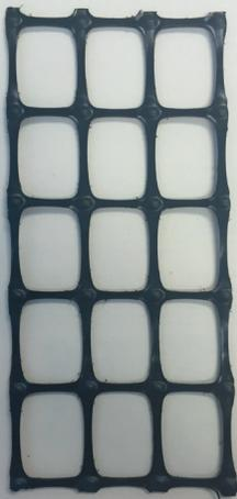
Simple, rectangular-shaped geogrid stabilizes aggregate and improves pavement resiliency.
