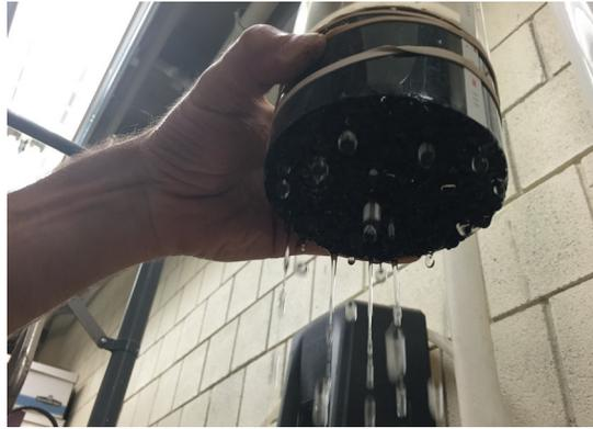
Pothole repair samples performed poorly in water penetration tests, which suggested that most mixes will perform poorly under seasonal freeze-thaw stresses.
