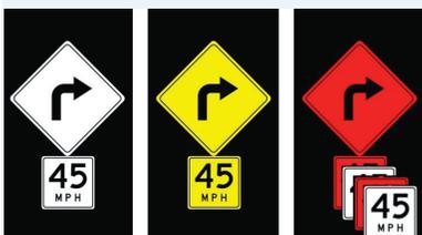
Researchers tested many curve warning sign progressions to determine which option drivers would most quickly understand.
