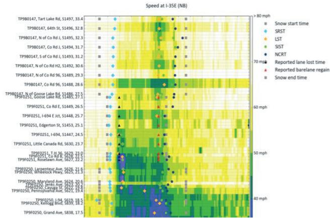
This speed contour map generated by the NCRT system shows the start of a snow event (gray squares), changes in traffic speed flow and reported bare lane regain times on I-35E northbound. Greater density of traffic appears in green and blue: Traffic speed on many roads was 40 mph or below soon after the snow began.
