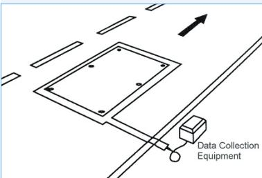
The NCRT system uses traffic flow data from loop detectors embedded in Minnesota highways.
