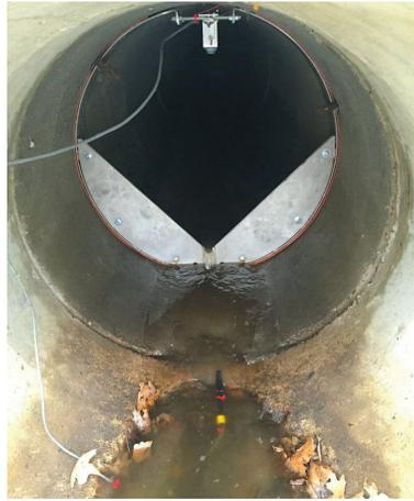
A V-shaped weir to measure flow was inserted into the bottom of this discharge pipe opening along County Road B. A depth monitor was mounted at the top. A conductivity monitor, located in the water beneath the weir, collected data that allowed researchers to determine chloride ion levels.
