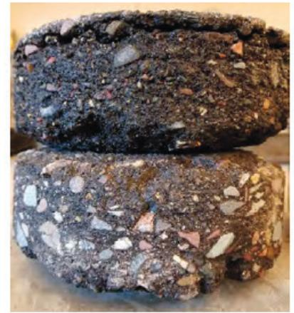
The samples above show an intact asphalt core (left) and a stripped core (right) under chip seal and between asphalt lifts that were collected from a site in Shoreview, Minnesota.
