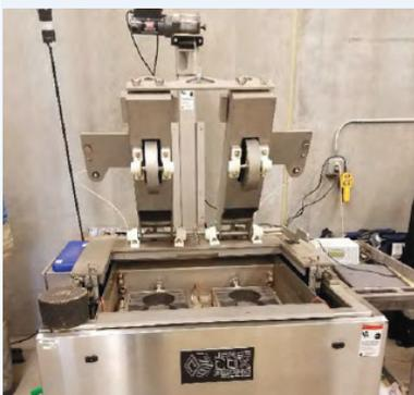
The Hamburg wheel track test reveals weaknesses in asphalt mixes, such as loss of adhesion between binder and aggregate.
