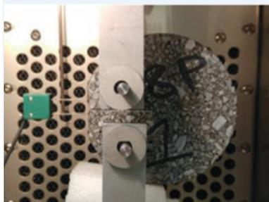
The disk-shaped compact tension test determines fracture energy of pavement samples, a strong predictor of cracking performance.
