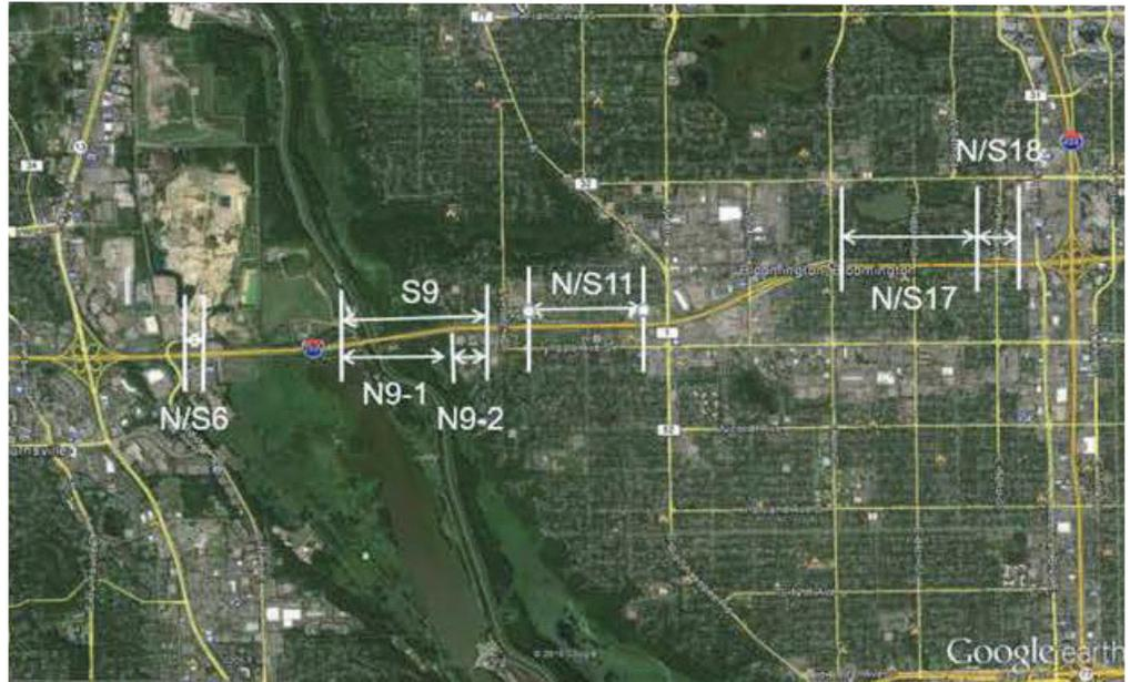
The HOT region segment contained sections with loop detectors that provided statistical analysis used in the study.
