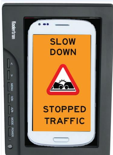
A smartphone was replicated through installation of an LCD screen positioned inside the driving simulator.
