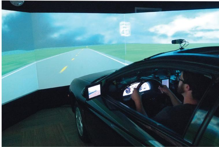
Drivers who participated in the study operated a 2002 Saturn SC2 complete chassis-driving simulator, which provided realistic control feedback through brake power assistance and resistance-based steering.
