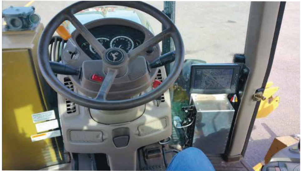
Mechanics constructed a metal rack to house the AVL unit (at right) within the cab. This location allows for convenient driver interface.
