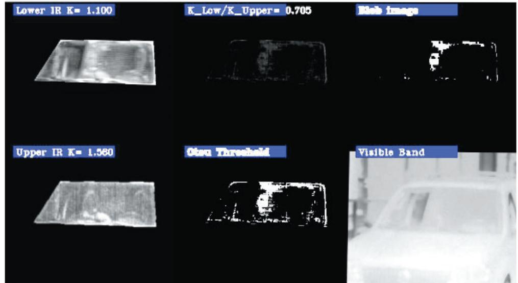
In outdoor tests without supplementary illumination, the sensor was able to detect a passenger through vehicle glass in only one case out of 24 attempts. With illumination, the sensor generally did not successfully detect a person through windshield glass.
