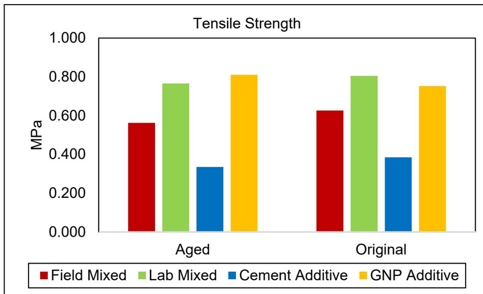
**Figure 7: Tensile strength for aged and original materials**
