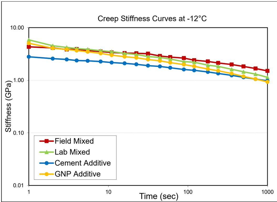
Figure 2: Creep stiffness curves at -12°C for all materials
