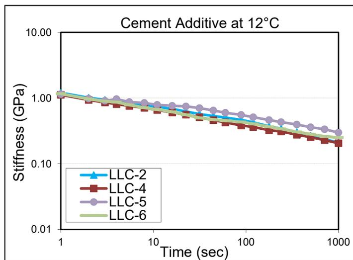
Figure 23: Creep stiffness curves for cement additive samples, at -12°C, 0°C and 12°C
