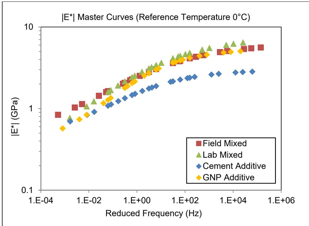
Figure 6: Fitted dynamic modulus master curves for all materials
