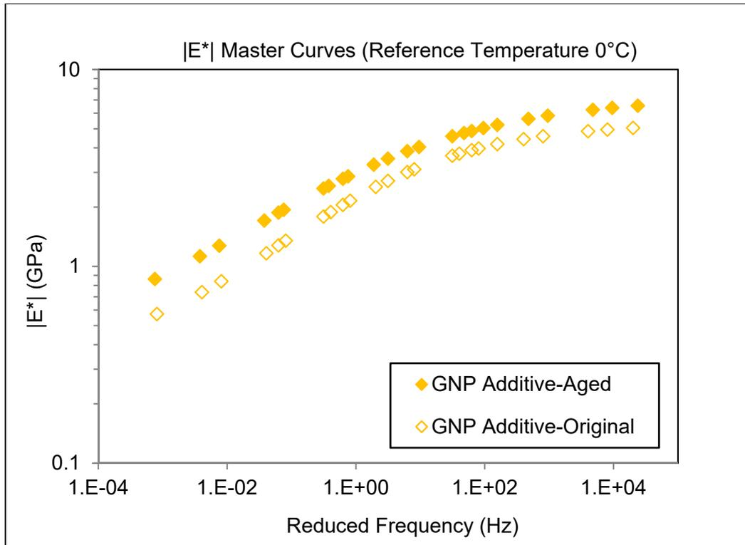
**Figure 11: Fitted dynamic modulus master curves for all GNP additive samples**
