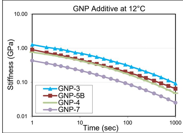
Figure 24: Creep stiffness curves for GNP additive samples, at -12°C, 0°C and 12°C
