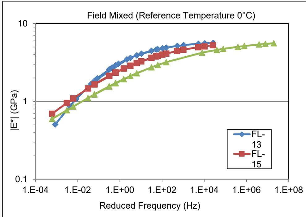
**Figure 25: Dynamic modulus master curves for field mixed samples.**
