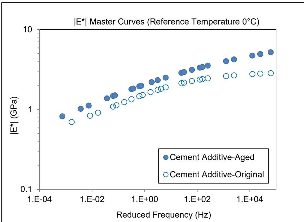
Figure 10: Fitted dynamic modulus master curves for all Cement additive samples
