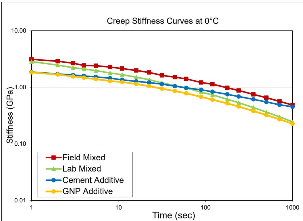
Figure 3: Creep stiffness curves at 0°C for all materials
