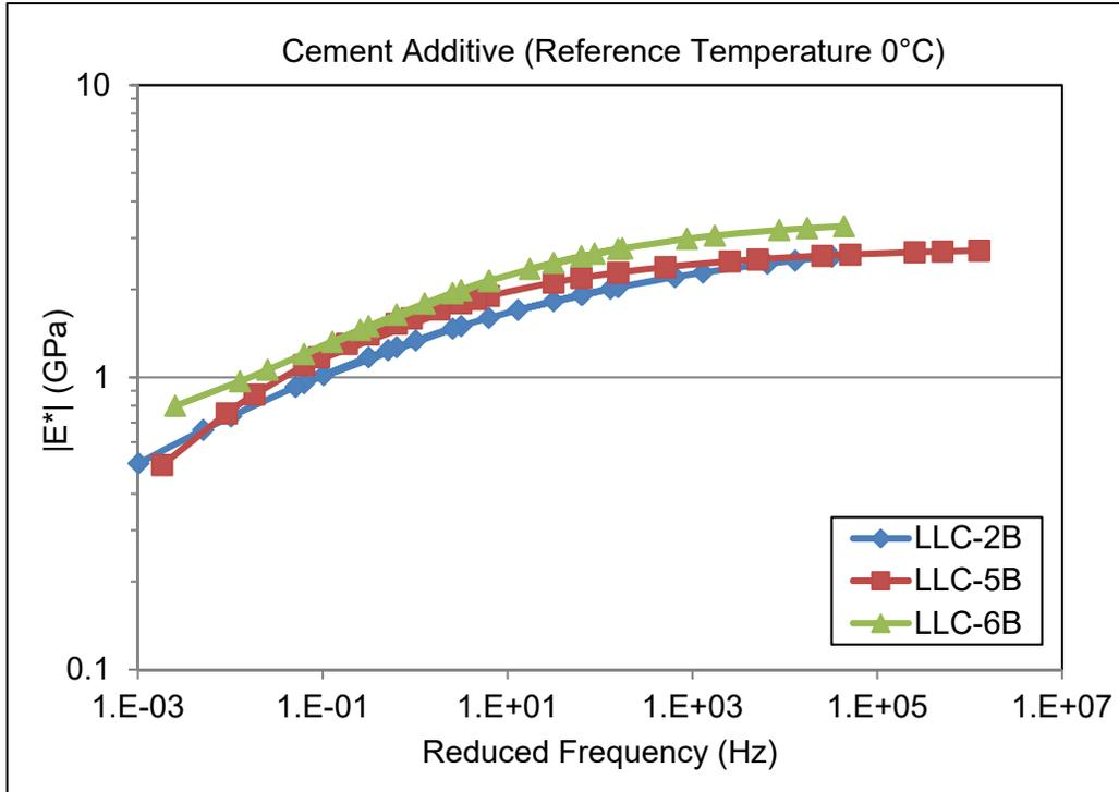
Figure 27: Dynamic modulus master curves for cement additive samples.
