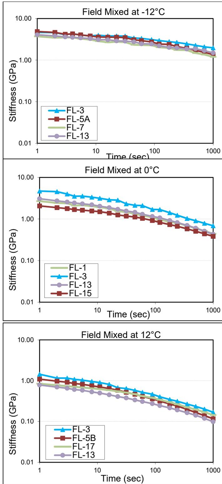
Figure 21: Creep stiffness curves for field mixed samples, at -12°C, 0°C and 12°C
