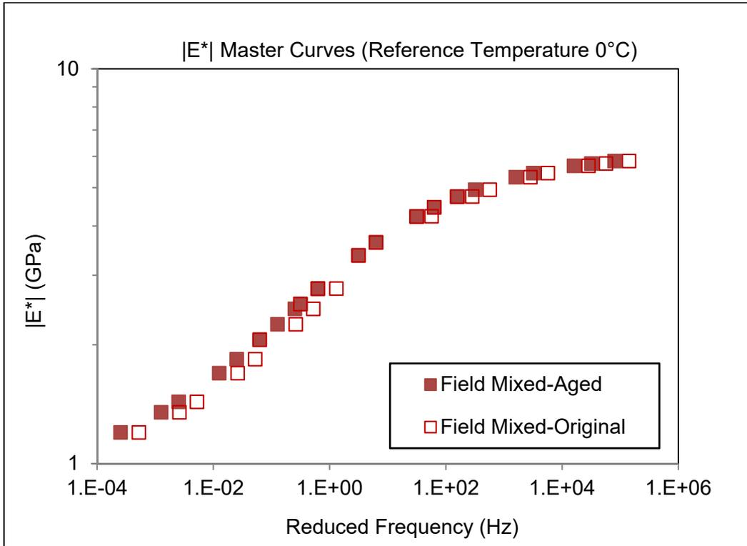
Figure 8: Fitted dynamic modulus master curves for Field mixed samples
