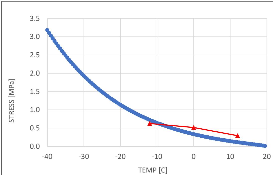
**Figure 14: Thermal stress and IDT strength results for lab prepared, lab compacted samples**
