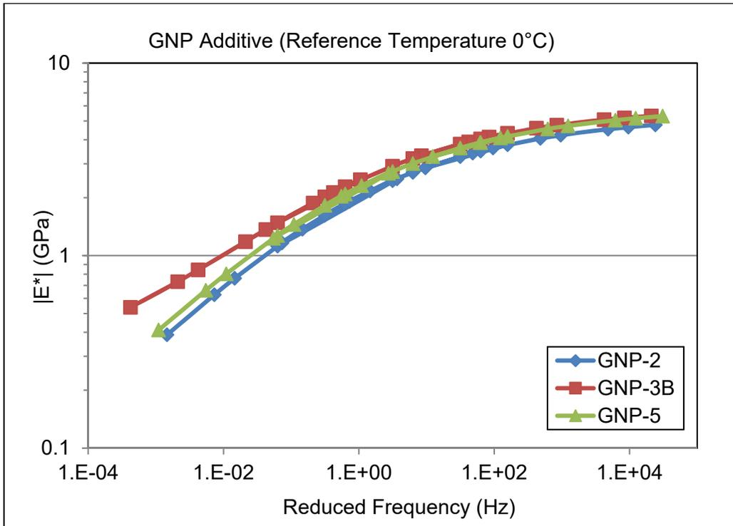
**Figure 28: Dynamic modulus master curves for GNP additive samples.**
