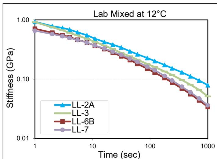
Figure 22: Creep stiffness curves for lab mixed samples, at -12°C, 0°C and 12°C
