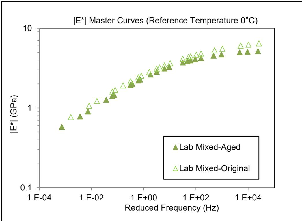
Figure 9: Fitted dynamic modulus master curves for Laboratory mixed samples
