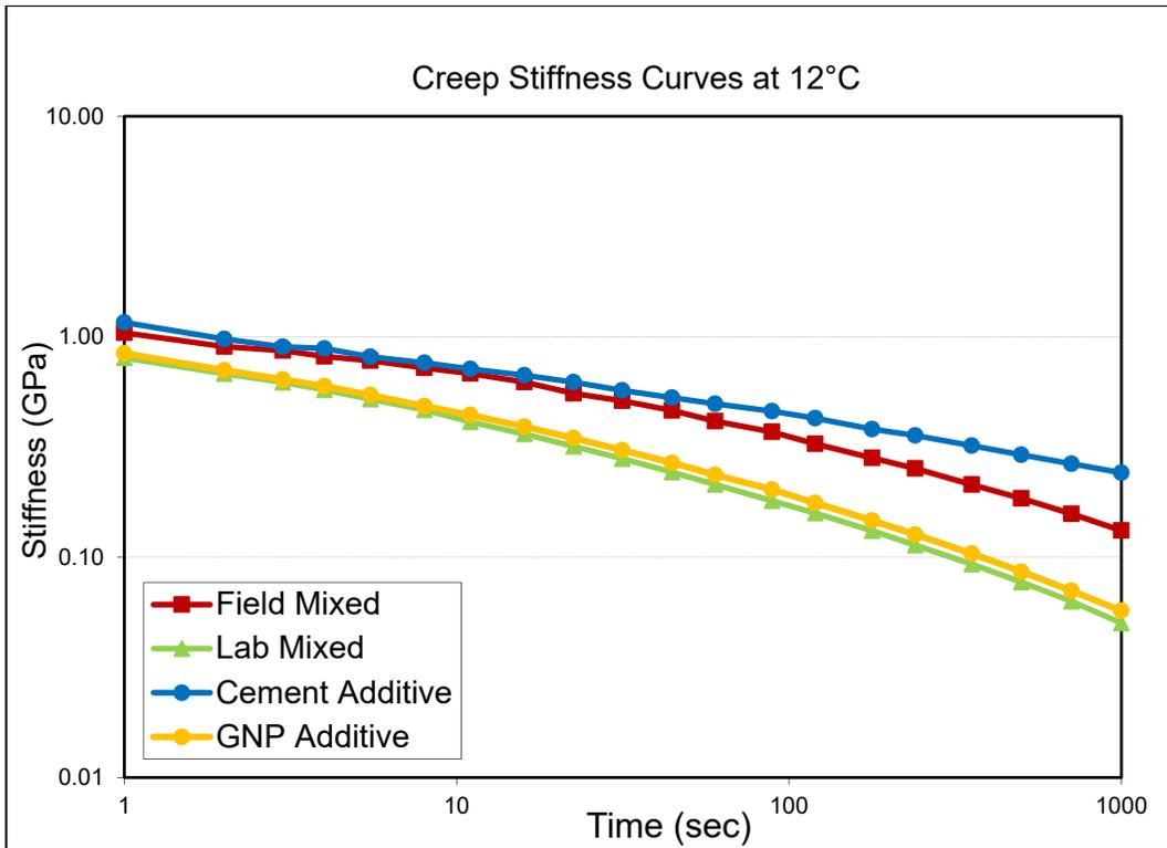
Figure 4: Creep stiffness curves at 12°C for all materials
