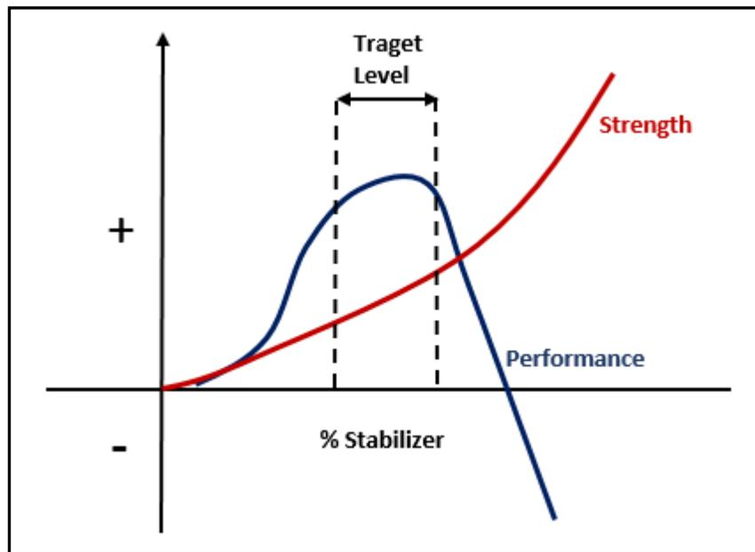
Figure 1: Balance between strength and performance for FDR stabilized with cement [3].
