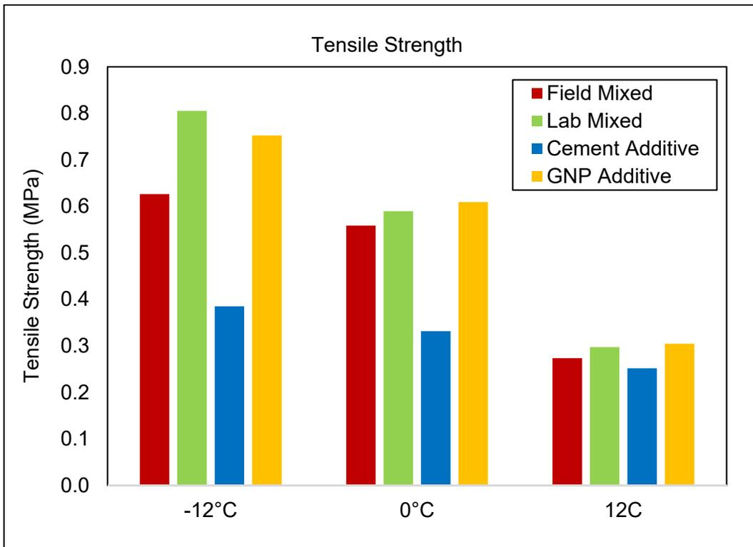
Figure 5: Tensile strength for all materials
