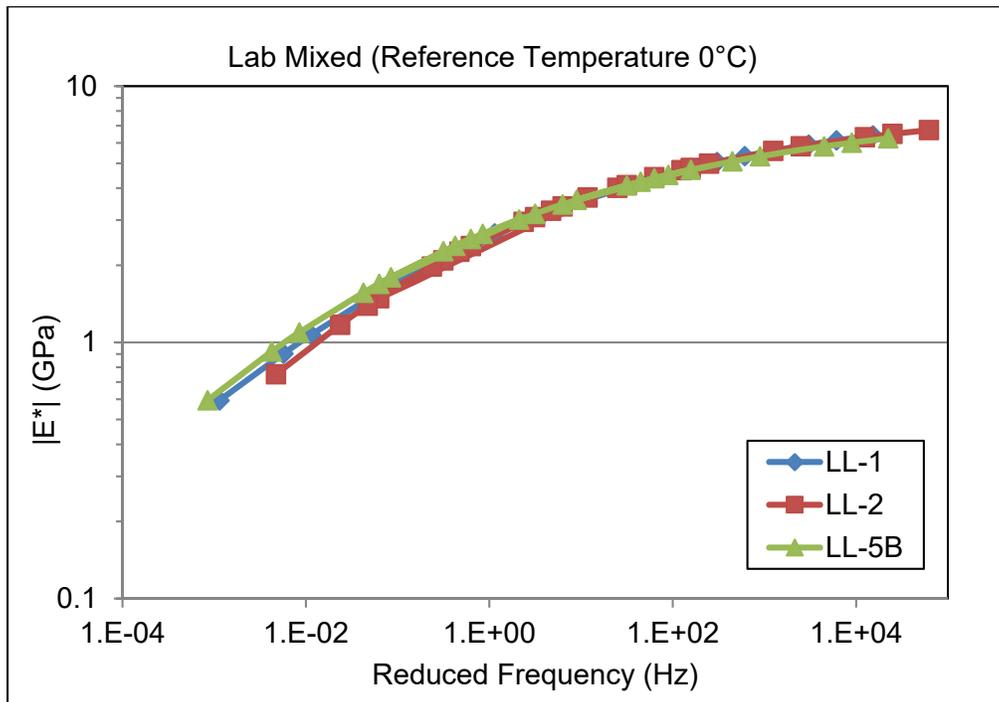
Figure 26: Dynamic modulus master curves for lab mixed samples.
